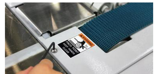
Access to belt and tape head changes for quick maintenance. Dekka has a deep support network all across North America
